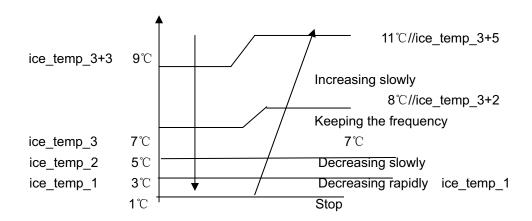
When Tpg\_indoor 〈 ice\_temp\_1, the frequency of the compressor decreases at the speed of 1HZ/1second.
