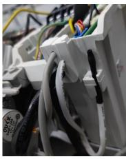
5. Install the housing and arrange the wiring harness to ensure that the front and rear buckle are installed in place.
